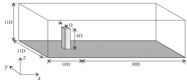
**Figure 3:** Computational domain of the fluid flow simulation;  $D = 20$  mm
