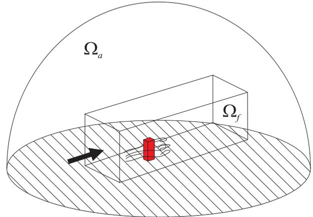
**Figure 1:** Schematic overview of the simulation setup divided into fluid domain  $\Omega_f$  and acoustic domain  $\Omega_a$
