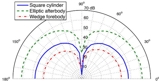
**Figure 4:** Directivity patterns of SPL in crossflow ( $yz$ -plane) for different geometries
