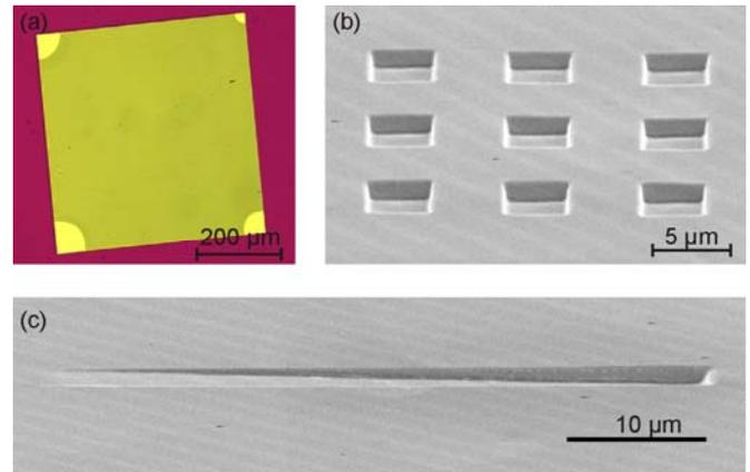
**Fig 1:** (a) Optical image of 30 nm thick membrane of silicon nitride, (b) SEM images of silicon membranes, and (c) trench structures.
