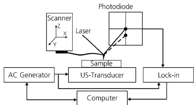
**Fig. 2:** Schematic of AFAM experimental set-up.
