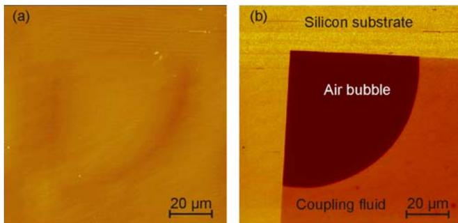
**Fig. 3:** (a) Topography and (b) AFAM amplitude image obtained for the 30 nm thick membrane of silicon nitride. The height scale of the topography image was 300 nm.
