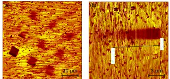
**Fig. 4:** AFAM images obtained for the (a) set of nine membranes and (b) trench structure with varying thickness.
