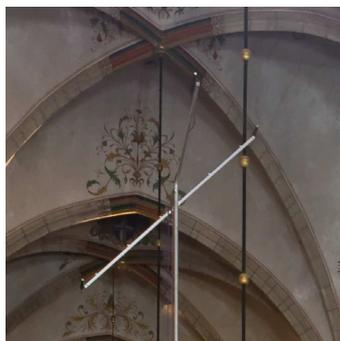
**Figure 1:** The configuration of the microphones trio at the acoustic documentation of the organ (method 8+1).
