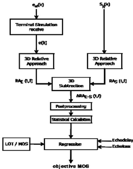
**Figure 4:** Block diagram of echo assessment model
