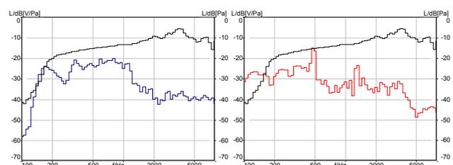
**Figure 3:** Sending frequency response (black) and power density spectrum (left (blue): female, right (red): male)
