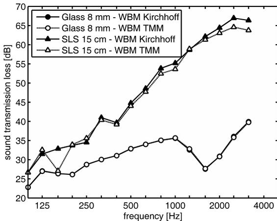
Figure 2: 8 mm glazing (1.25 m x 1.50 m) and 15 cm sandlimestone (3.05 m x 2.95 m), material properties Table 1.
