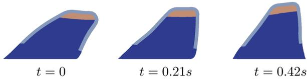
**Figure 4:** Three timesteps of the deformation generated using initial value with very low Young's moduli
