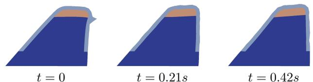
**Figure 6:** Three timesteps of the deformation generated using material parameters (see table 2) from the optimization with reference displacement from the hemilarynx experiment
