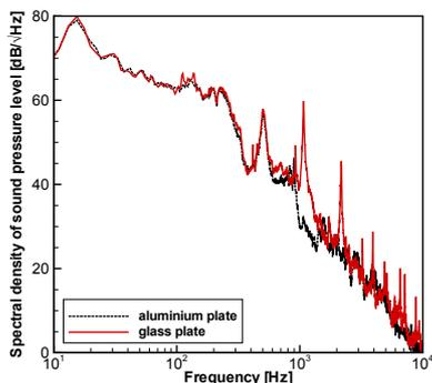
**Figure 5:** Sound pressure level at a 0.07 m distance perpendicular to the back side of the plates
