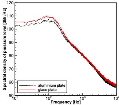
**Figure 4:** Frequency spectra of the wall-pressure fluctuations at  $x = 92$  mm and  $y = 0$  mm
