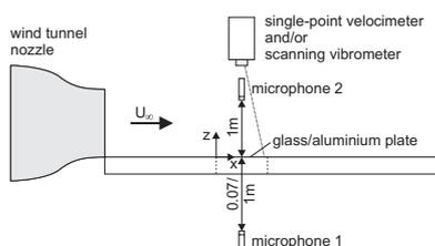
**Figure 2:** Sketch of the measurement setup, side view
