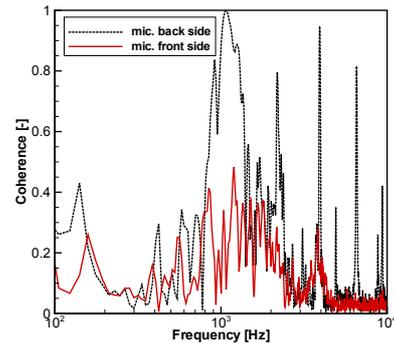
**Figure 6:** Spectra of the coherence between sound pressure signal (back side: 0.07 m distance, front side: 1 m distance) and plate velocity signal (centre point)
