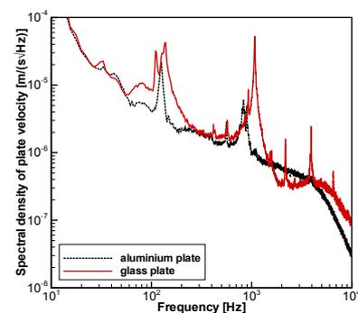
**Figure 3:** Frequency spectra of the measured vibration velocity in the centre point of the plates
