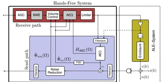
**Figure 1:** Block diagram of the proposed system. The receive path processing exploits PSD estimates available from the send path as well as the transfer function of AEC filter.
