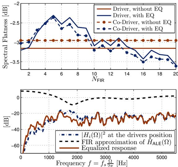
**Figure 2: Top:** Average spectral flatness as a function of the equalizer filter-order  $N_{\text{FIR}}$  for the driver and co-driver position. The spectral flatness may be increased with a low-order FIR approximation of Eq. 2. **Bottom:** Example frequency responses for  $i = 2$  and  $N_{\text{FIR}} = 5$ .
