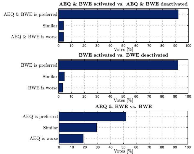
**Figure 3: Results of the subjective evaluation. Top:** Proposed system versus the reference (AGC, volume control and Limiter). **Middle:** AEQ deactivated versus reference. **Bottom:** Direct comparison AEQ & BWE versus BWE.
