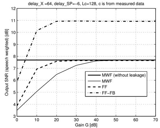
Figure 3: Performance comparison for MWF (with/without leakage) and ANC motivated algorithms
