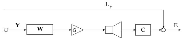
Figure 1: Hearing aid configuration with leakage
