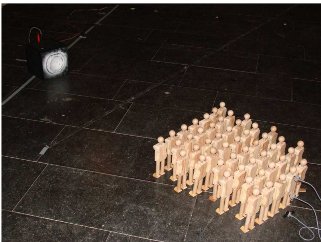
Fig 1: A scale measurements setup consisting of fifty 1:10 wooden models people, a loudspeaker and three microphones, which can be placed on different distances from the loudspeaker.
