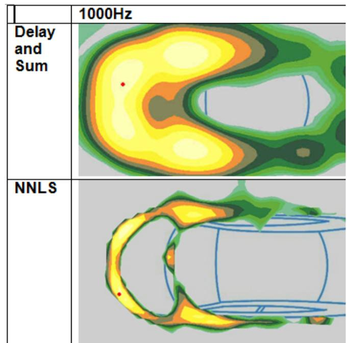
**Fig.1:** Wheel array supported above test vehicle in windtunnel. Top row: delay and sum results; bottom row: NNLS (Non-Negative Least Squares) deconvolution results. Display range 15dB.
