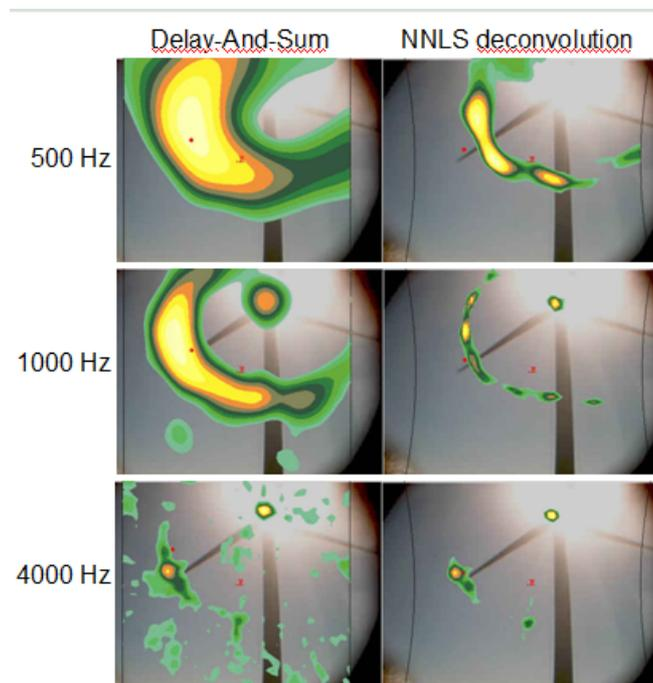
**Fig 3:** sound maps made down stream using a portable pentangular array. Delay and sum Beamforming results are on the left, NNLS deconvolution results on the right.
