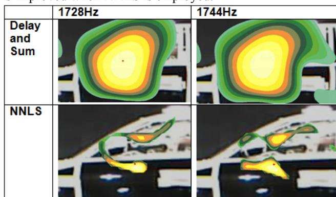
**Fig.2:** sound maps are shown for noise in 16Hz bandwidths. Virtually no difference is noticed for the Delay and Sum results whereas the NNLS shows considerable frequency related detail..
