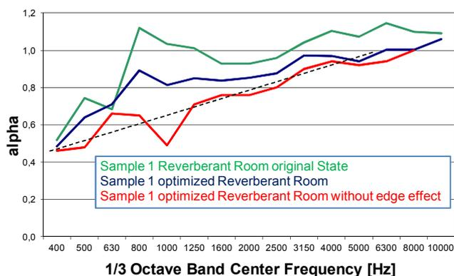
**Picture 4:** Measurement of one sample measured at different states of optimization. Green curve: before optimization, blue curve: with sound-deadening diffuser, red curve: with sound-deadening diffuser and without edge effect
