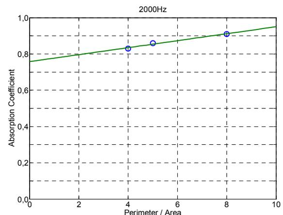
Picture 3: Elimination of the edge effect, by changing the ratio of perimeter/area the absorption coefficient can be found at 0 of the abscissas (here 0.76).
