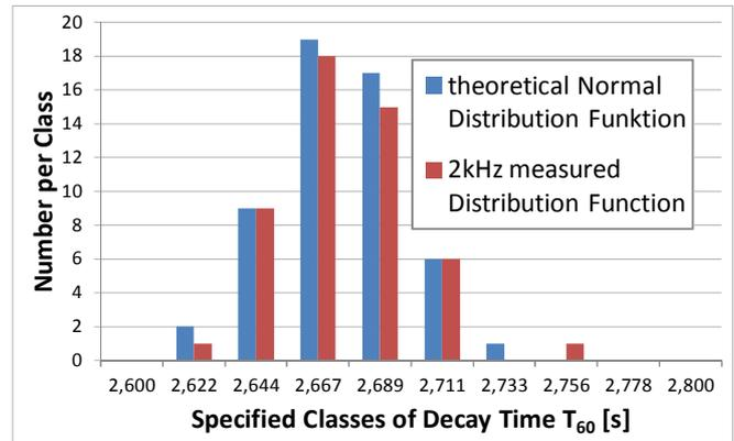
Picture 2: Theoretical and measured distribution function of the decay time at 2kHz tierce of one microphone position.
