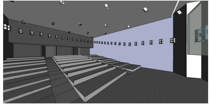
Figure 3: Loudspeaker arrangement in cinema
