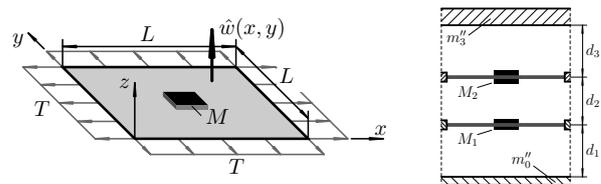
**Figure 1:** Left: Geometrical definitions of a square membrane centrally loaded with a rigid square mass. Right: Basic structure of a noise-shield design involving membrane layers.
