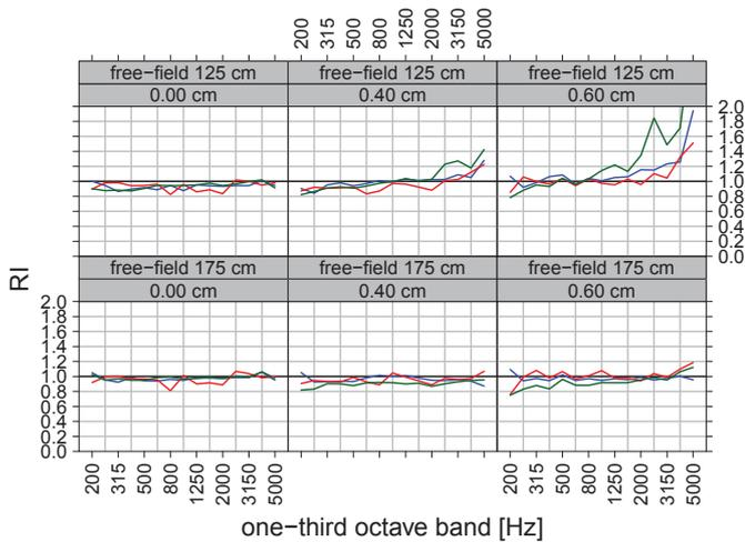
**Figure 2:** Reflection Index in one-third octave bands for three sound sources with different directional characteristics; upper row: without correction for directivity; lower row: with correction for directivity
