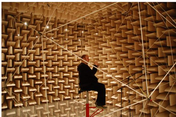
**Figure 2:** Spatial recording of a trumpet using a spherical array of 32 microphones in TU-Berlin
