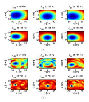
Figure 3: Objective functions at 185Hz (a) and 744Hz (b). State-of-the art objective function (top row) vs. proposed objective function (bottom row). Values represented in x-y, y-z and x-z planes in the left, middle and right columns, respectively.
