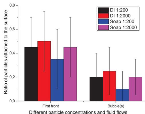
**Figure 4:** Ratio of particles still attached to the glass slide after the action of the first front and after subsequent bubbles loaded with particles. 1:200 and 1:2000 indicate slides contaminated with particle solutions diluted to this concentrations from stock solution. DI indicates the fluid was just DI water. Soap indicates the fluid was DI water with soap.
