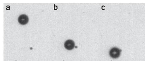
**Figure 2:** Experiment 1. (a): Bubble driven at 20 kHz and attached to the glass drifts downwards and attracts a particle by micro-streaming without being in direct contact before detachment. (b): The particle sticks to the bubble wall and is transported along with it (c).
