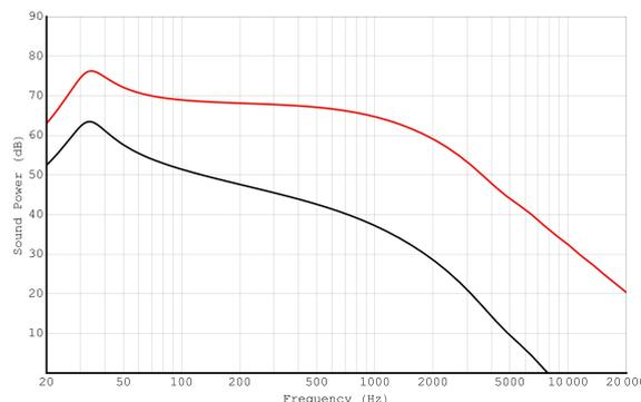
**Figure 2:** Sound power level of a 0.1 kg piston. Red line: tonal excitation at  $U = 1$  V. Black line: Pink noise with  $U_{tot}=1$  V.
