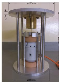
**Figure 1:** Teflon piston attached to a shaker. The piston moves inside a cylinder to avoid tilting motions. The creme colored foam material decouples the shaker from the aluminum bearings that connect the bottom and top plate.
