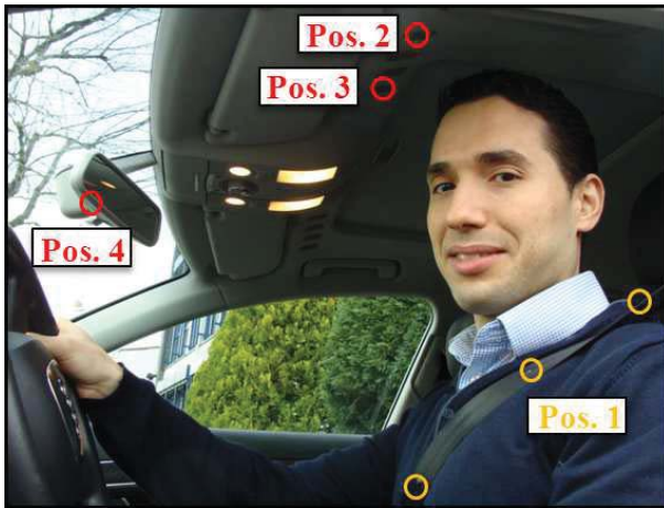
Figure 1: Belt-microphones (Pos. 1) and microphones positioned at the roof and at the mirror (Pos. 2 – 4).
