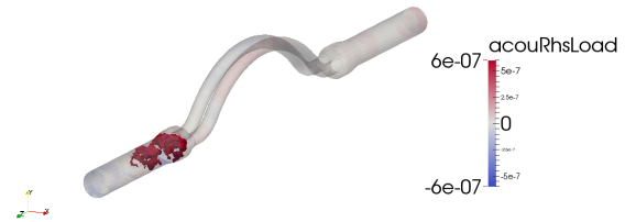
Figure 5: A contour plot showing the location of the maximum amplitude of an example acoustic source term at the outlet.
