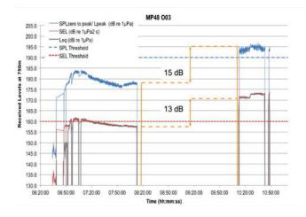
**Figure 1:** This graph shows time series of SEL (in red) and SPL (in blue) for the reference measurement. The noise mitigation screen was removed and an increase of 13 dB was observed for the SEL and 15 dB for the SPL
