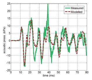
**Figure 2:** Example of near-field acoustic pressure time series at Anholt OWF from a single hammer impact, at 60 m range and 3 m off bottom for a pile penetration of 10 m: measured vs. modelled (WEAP-FE method).
