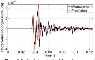
Figure 3 Predicted time signal of the underwater sound pressure in the near field and comparison with measurement data for Borkum Riffgrund 1. The corresponding  $\Delta$ SEL is 0.5dB.
