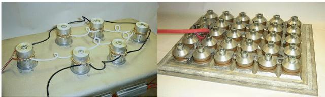
**Fig. 1: Examples of sound radiating areas with different transducer densities seen from downside.**
