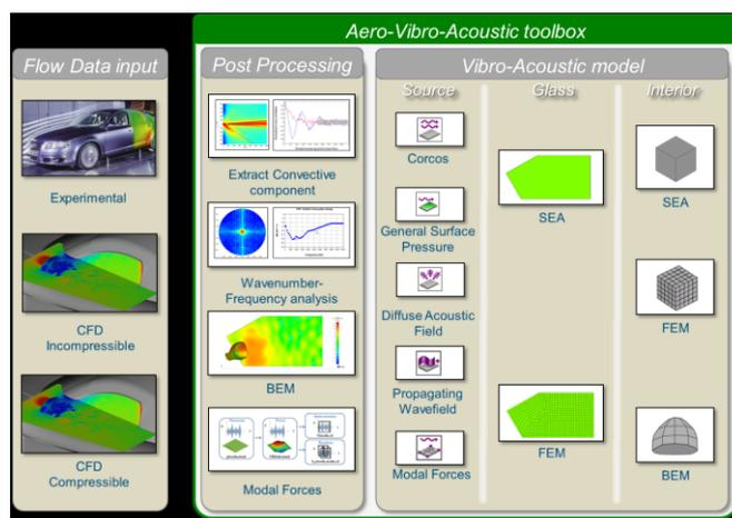
**Figure 1:** The overall workflow from surface pressure data to interior using different post processing techniques and vibro-acoustic models.
