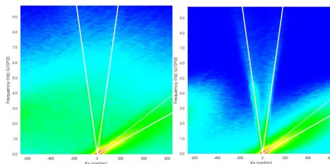
Figure 4: Wavenumber-frequency plots for nearest neighbour node (left) and conservative mapping operator (right).
