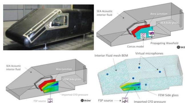
Figure 5: Photo of SAE body and pictures of vibro-acoustic models
