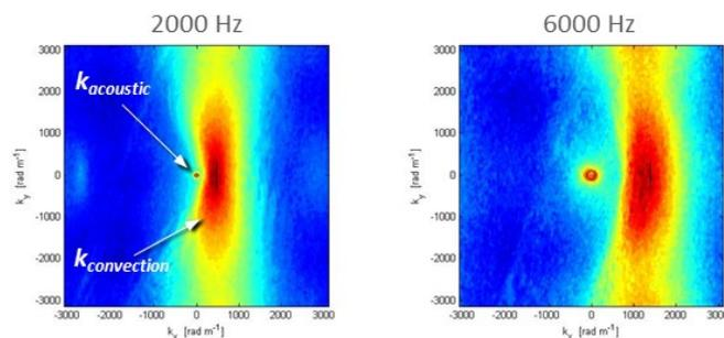
**Figure 2:** The wavenumber – wavenumber map of fluctuating surface pressure for 2000 Hz and 6000 Hz
