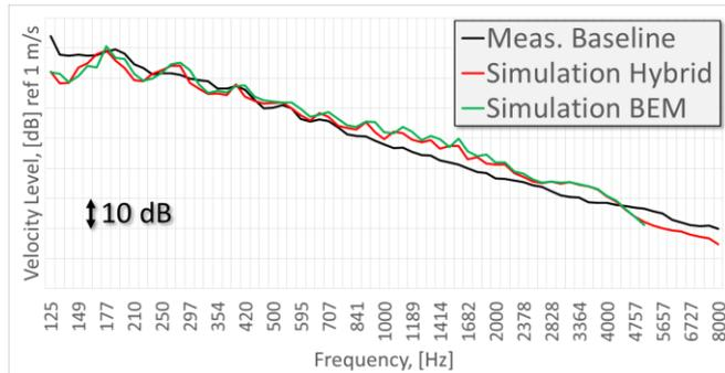
**Figure 6:** Average vibration of the FE side glass excited by modal forces
