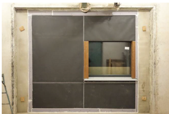
Figure 4: Test specimen consisting of 3 standard panels and 1 panel with window.
