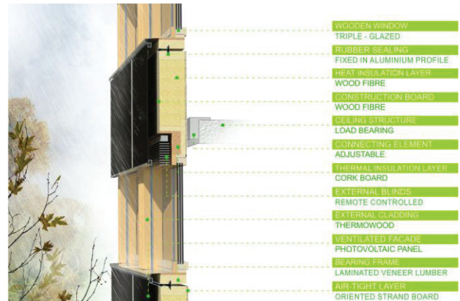
Figure 1: Scheme of the curtain wall consisting of wood-based panels [4].
