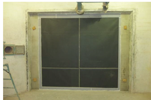
Figure 2: Test specimen consisting of 4 standard panels.
