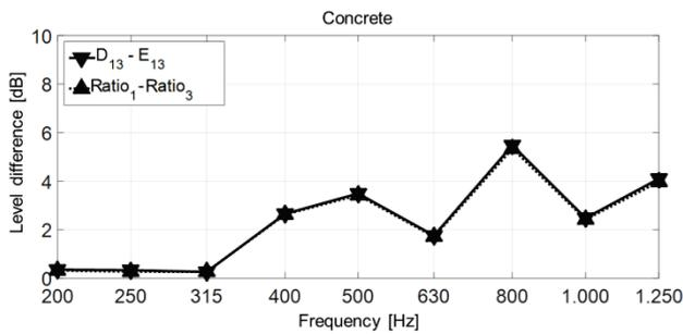
**Figure 8:** Correlation between deviation of velocity and energy based level differences and wave conversion (concrete)
