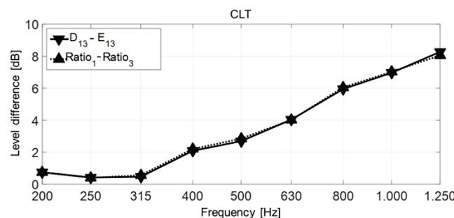
Figure 7: Correlation between deviation of velocity and energy based level differences and wave conversion (CLT)
