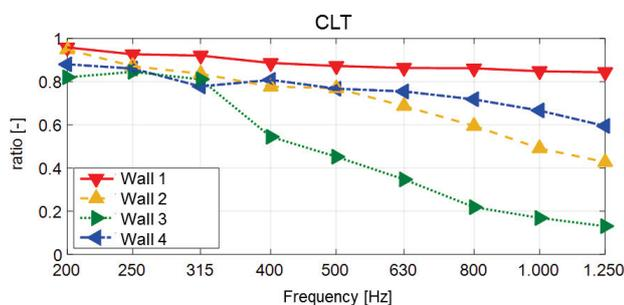
Figure 3: Ratio of out-of-plane components to the sum of out-of-plane and in-plane components (CLT)
