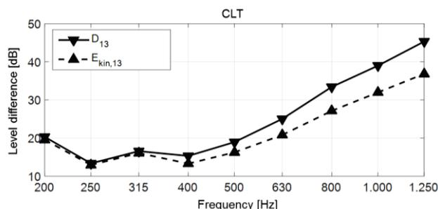
Figure 5: Velocity level difference compared to the level difference of the total kinetic energy density (CLT)
