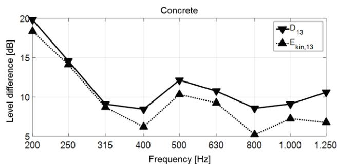
Figure 6: Velocity level difference compared to the level difference of the total kinetic energy density (concrete)
