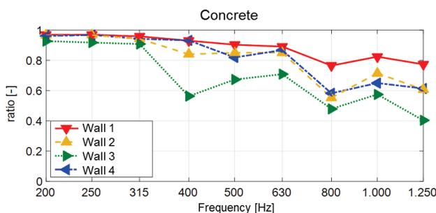
Figure 4: Ratio of out-of-plane components to the sum of out-of-plane and in-plane components (concrete)
