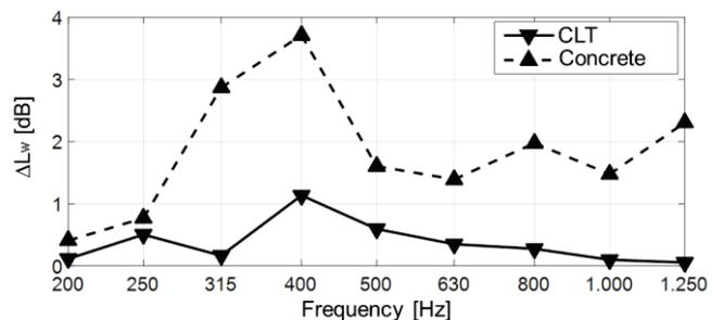
Figure 2: Contribution of sound radiation of wall 5 to the air-borne sound power of the receiving room
