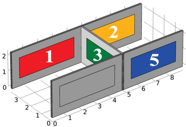
Figure 1: Geometry of the FEM model and area of spatial averaging of the velocities (CLT)
