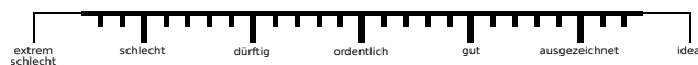
Figure 2: Continuous 7-point scale with German labels as used in the study. Translated labels left-to-right with MOS value: extremely bad (0), bad (1), poor (2), fair (3), good (4), excellent (5) and ideal (6).
