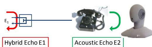
Figure 6: Setup for the determination of echo attenuation in a two-wire environment.
