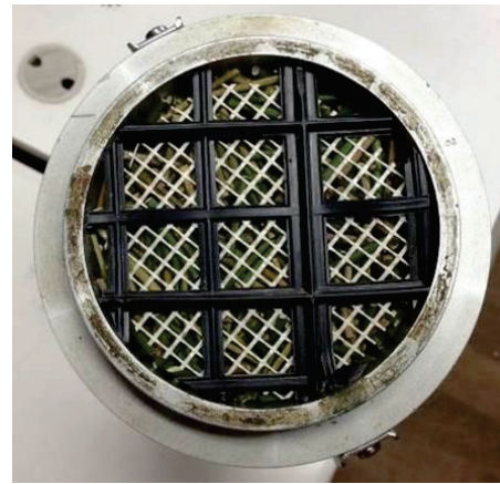
Figure 5: Loose broom in the Kundt's tube
