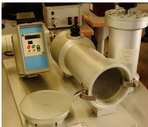
Figure 4: System for the measurement of the resistivity R_1 , with the method of the alternate air flow
