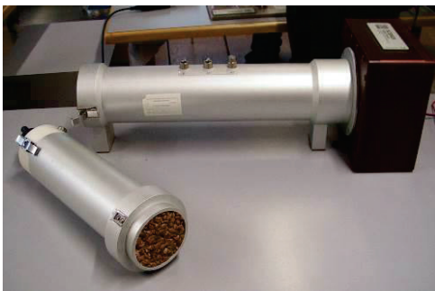
Figure 3: Tube of Kundt, for the absorption coefficient measurements
