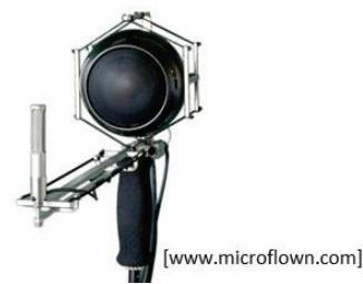
Figure 1: In-situ impedance measurement device from Microflown Technologies
