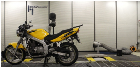
Figure 2: Laboratory test setup (II), HATS position close to motorcycle
