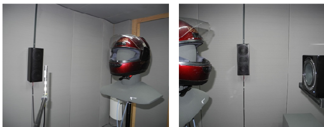
Figure 3: HATS with mounted helmet for tests in sending (left) and receiving direction (right)
