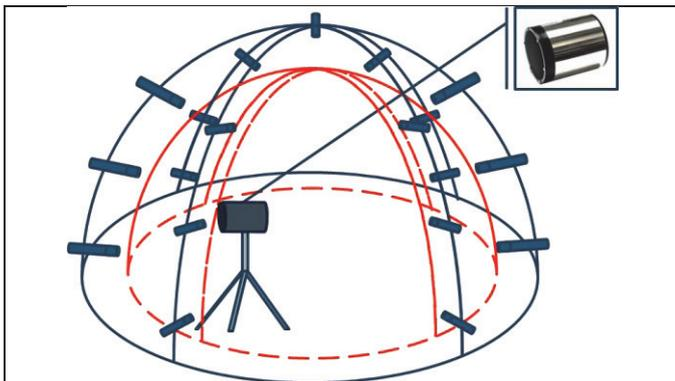
**Figure 1:** Experimental setup: loudspeaker fixed on a tripod, blue frame: hemispherical setup with 19  $\frac{1}{4}$  inch microphones, red dashed frame: the assumed shape of the studied source.
