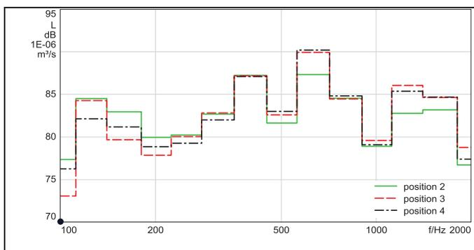
**Figure 11:** Predicted  $Q$  for loudspeaker 2 at position 2-4 for low correlation between signal 1 and signal 2.
