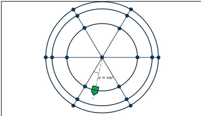
**Figure 3:** Changing the volume velocity position: top view of the measurement setup. Blue dots: positions of the microphones, green pentagon: position of the volume velocity source.
