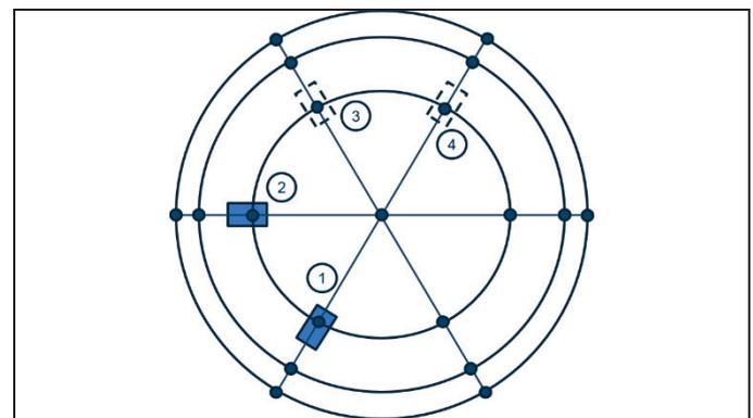
**Figure 6:** Experimental setup: two loudspeakers fixed on tripods: loudspeaker 1 always positioned at position 1, loudspeaker 2 at positions 2, 3, and 4, successively.
