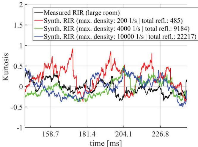
**Figure 3:** Normalized kurtosis evaluation for four RIRs of the large room. Evaluation is done with a sliding window (1024 samples) starting at 150 ms (Hidaka mixing time: 167 ms). Plot shows the curve for a measured RIR and three synthesized RIRs for three different maximum reflection density limits (200, 4,000, 10,000)
