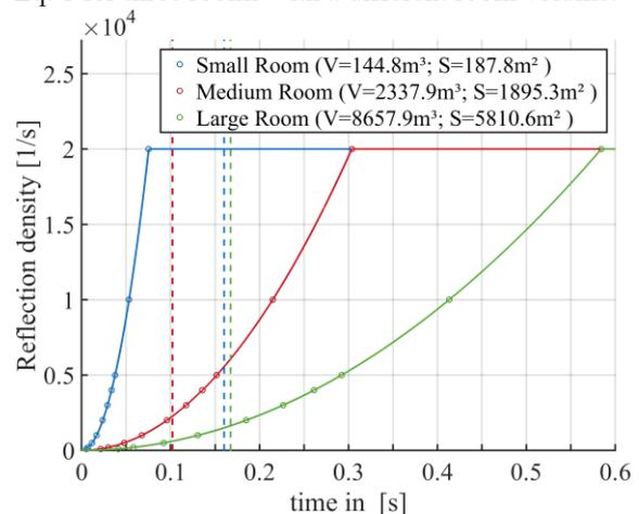
**Figure 2:** Reflection density function for different room sizes, with a maximum reflection density of 20,000 1/s. Dashed lines show the Hidaka mixing time for each room.
