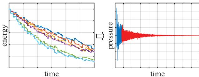
**Figure 1:** From energy histograms for separate frequency bands to broadband room impulse response.
