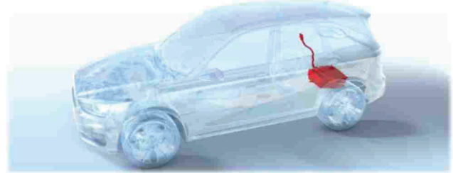
Figure 1: An SCR tank in the typical position in a vehicle.
