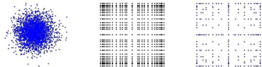
Figure 6: Collocation point selection strategies in 2D space: Monte Carlo simulation (left), full tensor grid using Clenshaw-Curtis quadrature (middle), Smolyak's sparse grid using Clenshaw-Curtis quadrature (right).
