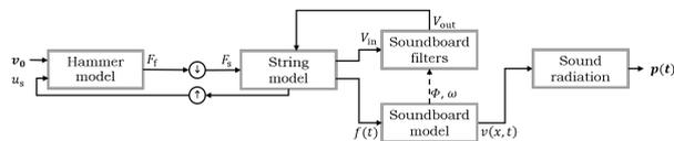
**Figure 2:** The block diagram of the piano model.
