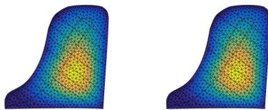
**Figure 9:** The first modes of the soundboard in deterministic (left) and stochastic (right) cases.
