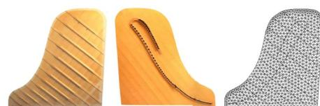
Figure 7: Used soundboard model: 1.50 m, 13 ribs, 1 curved bridge.
