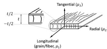
Figure 3: The laminated material model.
