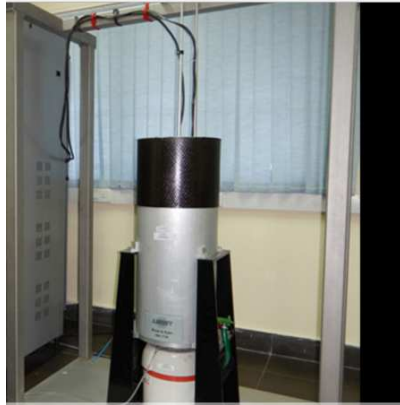
Figure 4: The test vessel is a thick walled \varnothing 300 mm aluminum tube with a vibrating bottom. The remaining instrumentation and the PC is in a nearby rack.
