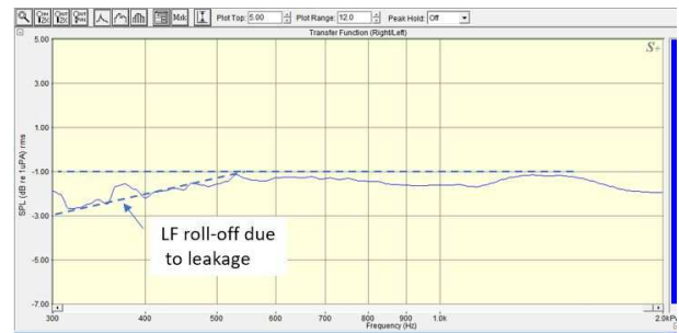
Figure 11: Measured response of a hydrophone with excess LF roll off due to leakage in the hydrophone.
