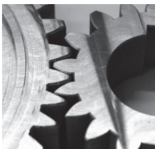
Figure 1: example of an inequidistant gearing with irregular tooth thicknesses and pitches
