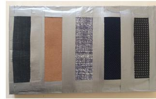
**Figure 1:** Textures used at the experiments: From left to right: Denim, cotton, canvas and automobile seat textile 1 and 2.
