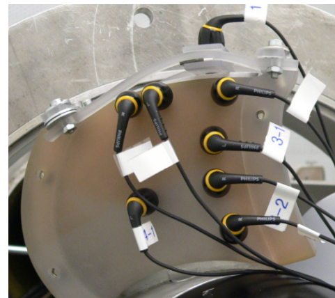
Fig. 1: Miniature microphones on a fan blade (top) and in-situ calibration with pre-calibrated headphones on a clamp-on adapter (bottom), from [1]
