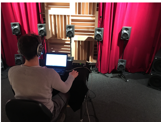
Figure 5: Listening Test Setup in the Immersive Media Lab.
