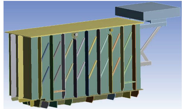
Fig 8: Transformer tank with additional optimized diagonal stiffeners
