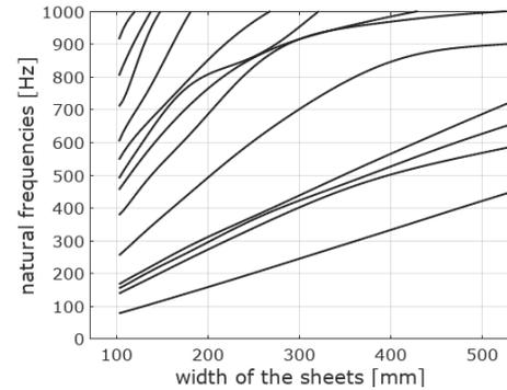
**Figure 5:** natural frequencies of different mode shapes versus the sheet width  $BB$
