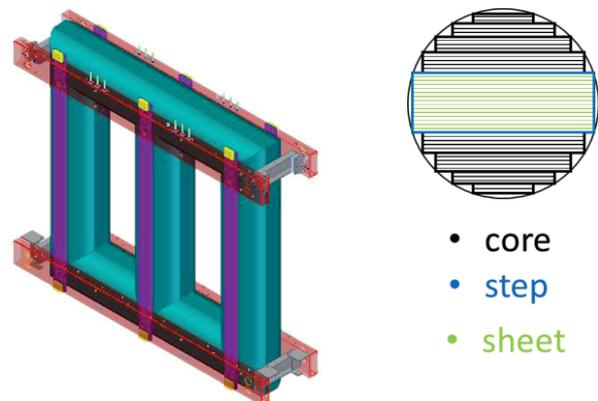
Figure 1: Transformer core
