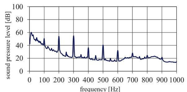
Figure 3: No-load noise measurement example
