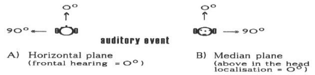
FIG. 2: Comparison of auditory events using a HFI (A), and a common headphone (B).
