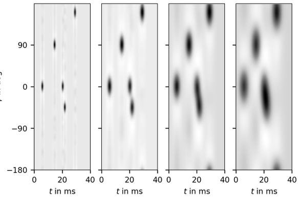
(b) Pre-processed PWD filtered by multiscale Gaussian kernel.
