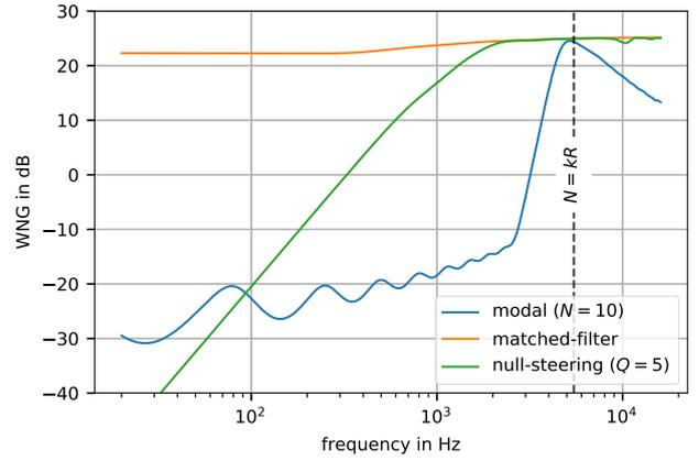
**Figure 3:** White-noise gain (WNG) of a modal, matched filter and null-steering beamformer (rigid array,  $R = 0.1$  m,  $N = 10$ , Lebedev grid, modal order of simulated soundfield  $N_{sf} = 32$ ,  $\theta_{pw} = 90^\circ$ ,  $\phi_{pw} = 0^\circ$ , Tikhonov regularization  $\beta=0.01$ ).
