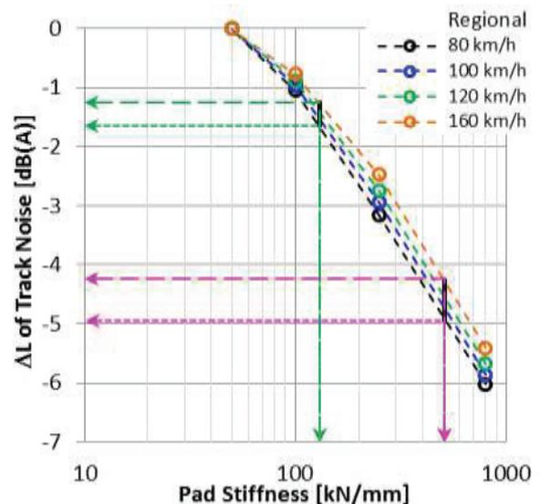
Figure 6: change in the radiated noise of disk braked regional trains at different speeds for soft (green lines  $s \approx 130$  kN/mm) and hard pad stiffness (purple lines  $s \approx 510$  kN/mm)
