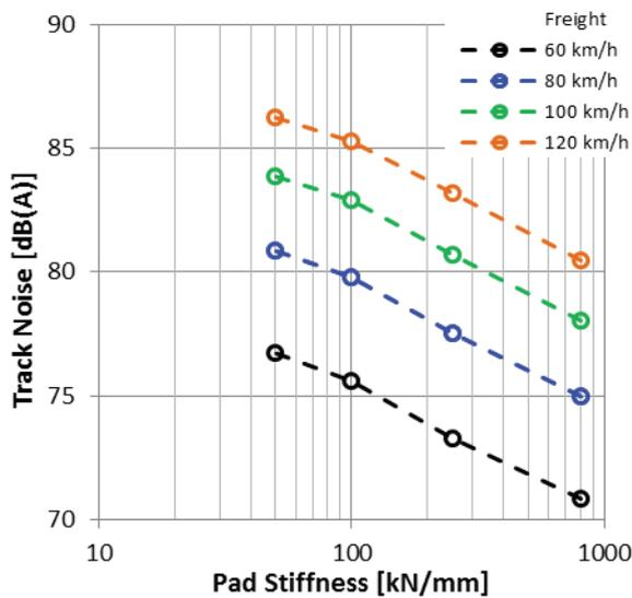
Figure 3: calculated noise levels of K-block braked freight trains at different speeds due to different pad stiffness; SPL at 7.5m beside track 1.2m above rail head
