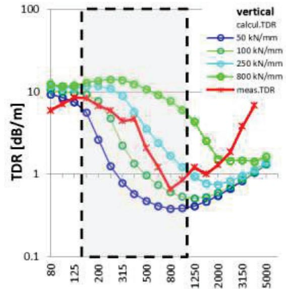
Figure 2: Calculated and measured TDR for vertical direction
