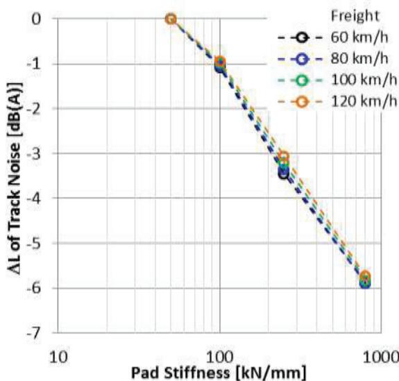
Figure 4: change in the radiated noise of K-block braked freight trains at different speeds normalized to pad stiffness of 50 kN/mm
