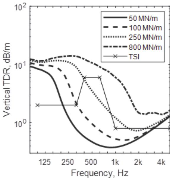
Figure 1: Examples of analytical calculations of TDR related to increasing pad stiffness
