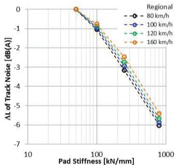
Figure 5: change in the radiated noise of disk braked regional trains at different speeds normalized to pad stiffness of 50 kN/mm
