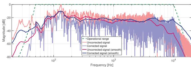
**Figure 11:** Comparison between corrected and uncorrected spectra (applying the inverse filtering).
