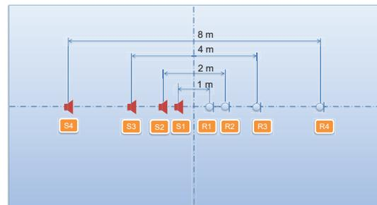
Figure 8: Measurement site with on axis source-receiver conditions (distances of 1 m, 2 m, 4 m and 8 m).
