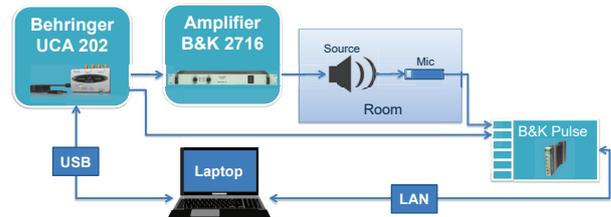
Figure 7: Measurement setup flowchart.
