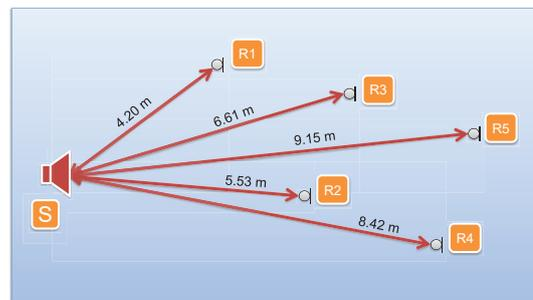
Figure 9: Measurement *in situ* in Room 355 (the sound source remained still in the position of the speaker and 5 receivers were configured in the chairs).
