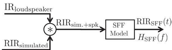
**Figure 2:** Overview of the SFF simulation. The sign “\*” denotes the convolution operation and the SFF block denotes the SFF method applied to the full  $RIR_{\text{sim.+spk.}}$ .
