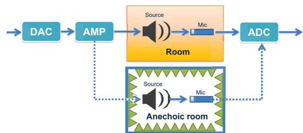
Figure 1: Typical measuring chain for RIR extraction.
