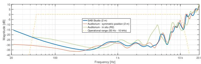
**Figure 10:** Frequency response of correction filters obtained from the three measurement conditions using dodecahedral sound source (B&K Type 4292).
