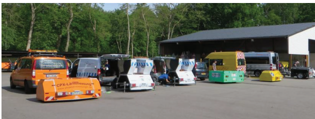
Figure 2: Preparation CPX-measurement systems for the round robin test 2017.
