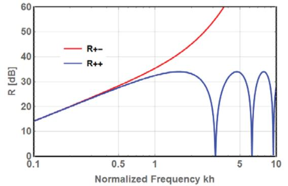
**Fig. 6:** Transmission loss of elastic layers with normalized impedance magnitude  $\zeta_L = 100$  between equal fluids. The signs of  $\rho_L$  and  $K_L$  are different for the curve  $R_{+-}$  and equal for the curve  $R_{++}$ .
