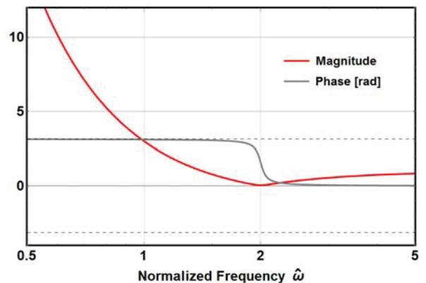
Fig. 2: Magnitude and phase of the normalized complex mass representing a harmonic oscillator.
