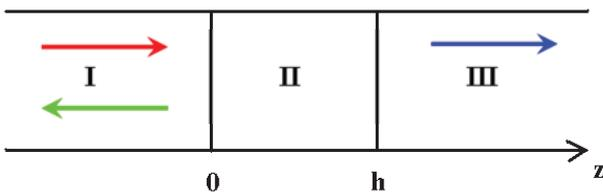
Fig. 1: One-dimensional sound transmission model with incident and reflected waves in region I, partition with thickness  $h$  in region II, and transmitted wave in region III.
