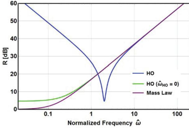
**Fig. 3:** Transmission loss of harmonic oscillators: with complex mass as in Fig. 2 (blue), with resonance frequency set to zero (green), and with damping set to zero as well, which leads to the usual mass law (purple).
