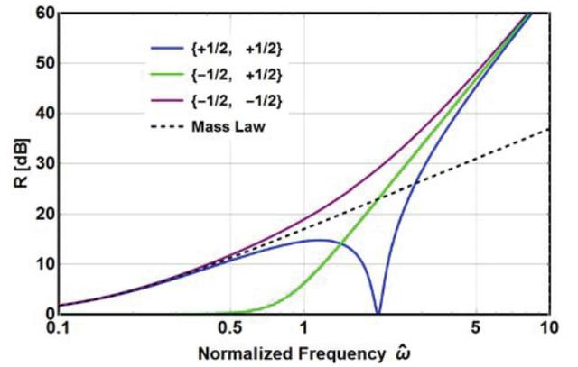
**Fig. 4:** Transmission loss of mass-spring-mass systems in air with stiffness  $\hat{C} = 1$  and masses of equal magnitude  $|\hat{M}_1| = |\hat{M}_2| = 1/2$ , but with different sign combinations. Dotted line: mass law for  $|\hat{M}| = 1$ .
