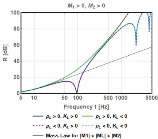
**Fig. 7:** Transmission loss of elastic layers sandwiched between two equal rigid positive masses for the four sign combinations of  $\rho_L$  and  $K_L$ . The black line shows the mass law as indicated in the legend.
