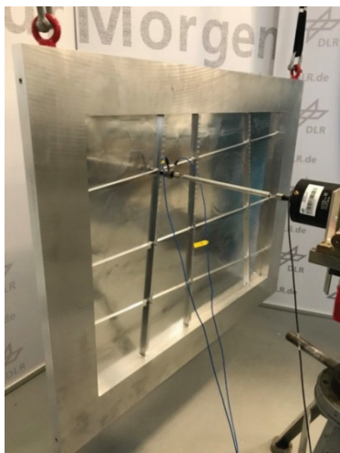
Figure 8: Aluminum plate used as test structure.
