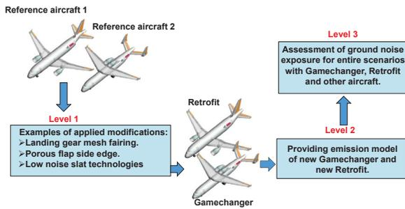
Figure 3: A schematic picture of the modification process applied on two reference aircraft in a three-levels framework.
