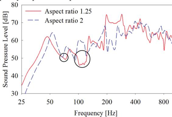
**Figure 6:** Frequency response for membrane aspect ratios 1.25 and 2 when exciter placed at 1/3<sup>rd</sup> of the length and width.
